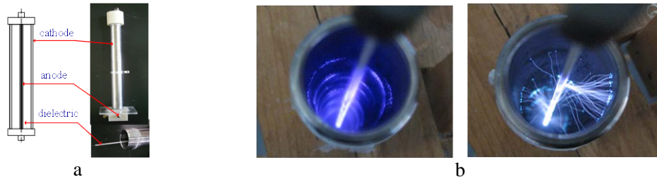
Figure 7. Generation of plasma discharges in DBD reactor: a) Reactor structure for plasma discharges in water; b) Physical characteristics of a DBPD in: helium (left) and argon (right)
